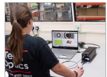
Interferometric end-face geometry check
