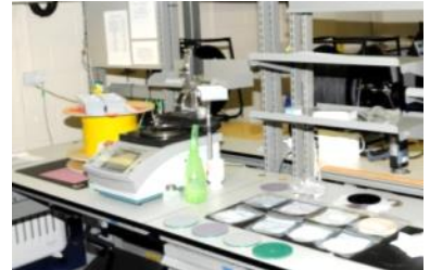
Tech Optics fibre optic polishing station
