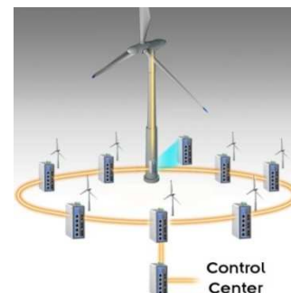
fig. 2 Fiber optic network for Wind Farms
