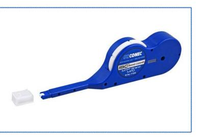
The MTP I.B.C. (In Bulkhead Cleaner) is the first dry cloth cleaner specifically designed to clean the MTP/MPO connectors while inside of an adapter, face-plate or bulkhead. The unique design enables cleaning of either male (with pins) or female (without pins) MT ferrules, single mode APC or multimode. This is an essential tool for networking equipment, such as switches and routers.
