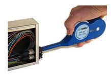
Cleaning 'behind the wall' with the Reel Cleaner inserted into an array adaptor.
