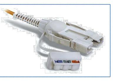
Taking advantage of the first network standard, designed from start to finish for fibre optics, the AMP Fixed Shroud Duplex (FSD) System offers the components necessary for a high performance FDDI local area network. The FSD connector, based on proven 2.5mm ceramic ferrule technology, is a two channel snap-fit connector that combines low loss, typically 0.2dB, with positive side latch mating, polarisation, easy to use keying and bend limiting strain relief.
